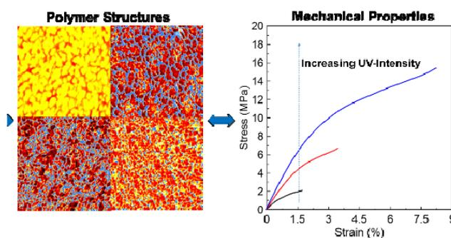
Figure 1, Polymer morphology and corresponding mechanical properties of hybrid radical/cationic systems with increasing UV curing intensity.
