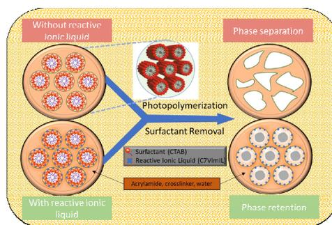
Figure 1: Representative LLC templating process used to generate a hexagonal nanostructure in organic polymers.
