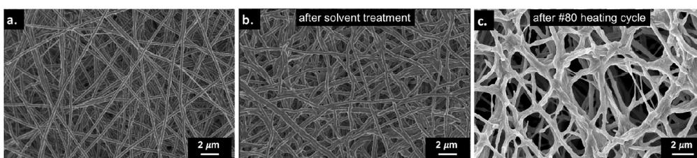
**Figure 1** FESEM images of **a.** crosslinked electrospun PEO membrane, **b.** after immersion in water, and **c.** after 80 heating/cooling cycles above PEO melting temperature.
