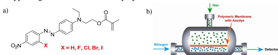
Figure 1. a) Scaffold of synthesized azodyes with different halogens in the ortho position respect to the azo group. b) Schematic representation of permeometer device.
