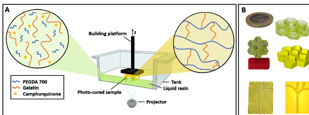
Figure 1: DLP printing scheme (A) and printed geometries (B).
