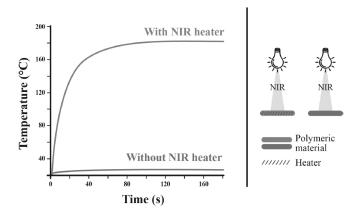
Figure 1. Photothermal effect of heater upon NIR light
