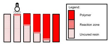
Figure 1: UV-induced frontal polymerization.
