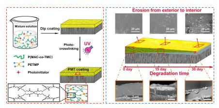
Scheme 1. Schematic illustration of the preparation of UV cured PMT coating on Mg alloy.
