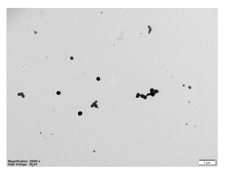
TEM micrograph of particles of PEG-HPMA copolymer prepared by photo-operated flow ATR-PISA without degassing in water.
