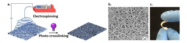
**Figure 1**. a: Scheme of the process, which couples a first electrospinning step and a subsequent photocrosslinking reaction. b: FESEM image of a rubber photo-cured electrospun mat. c: Picture of a photocrosslinked fibrous membrane showing its flexibility.
